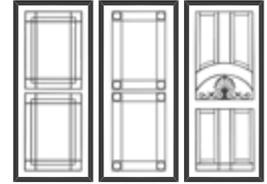
\*Panels are centre mounted on the mesh with a fixed vertical gap between the panels. This varies dependent on the selected panel. As the size of the door varies, the perimeter space will change.
